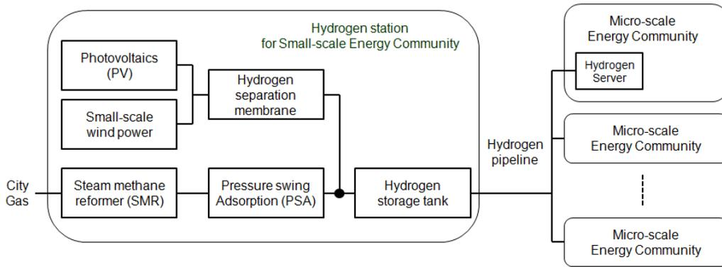
Fig. 8 Diagram of hydrogen station for Small-scale Energy Community
