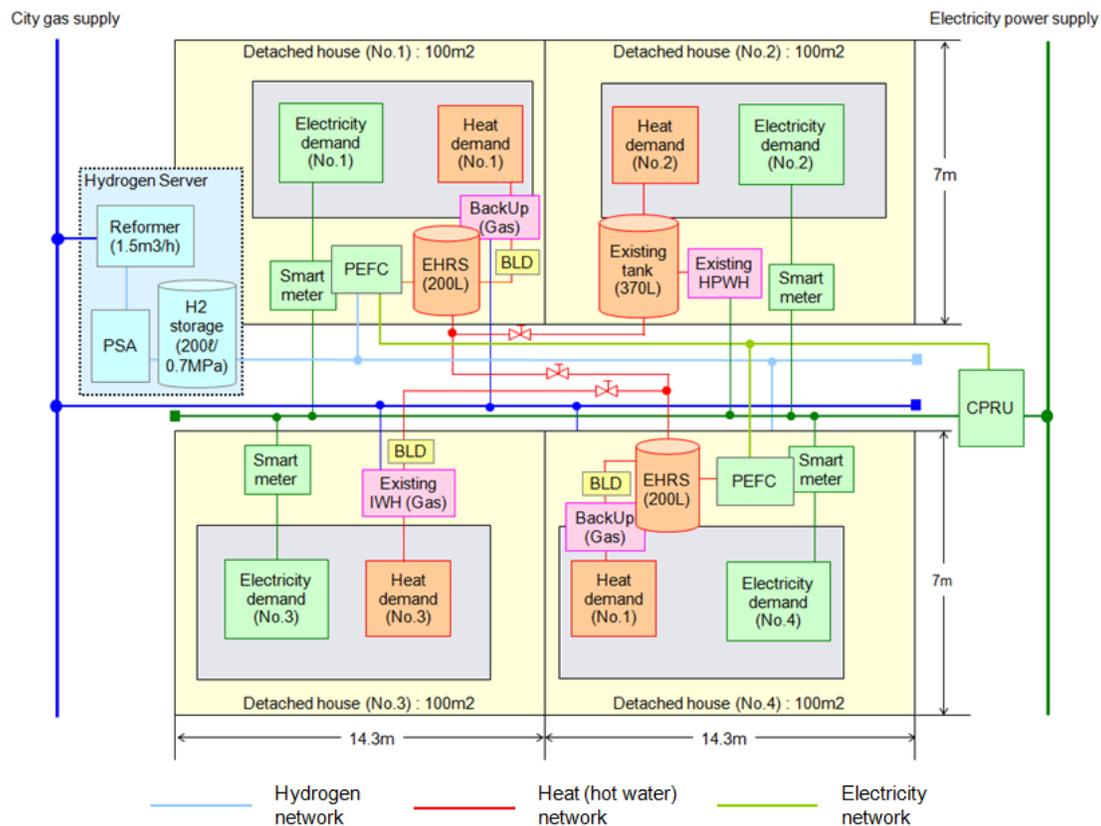
Fig. 5 Design example of four houses' network model
