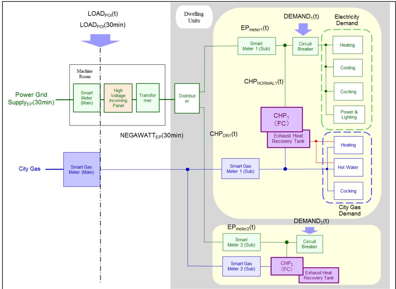
Figure 1. Energy networks of the model apartment building equipped with FCs and exhaust heat recovery tanks
