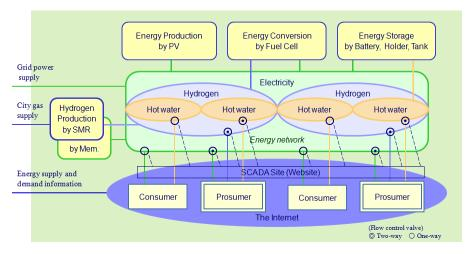
Fig. 1 Energy network topology of Hydrogen Energy Community balanced supply with demand
