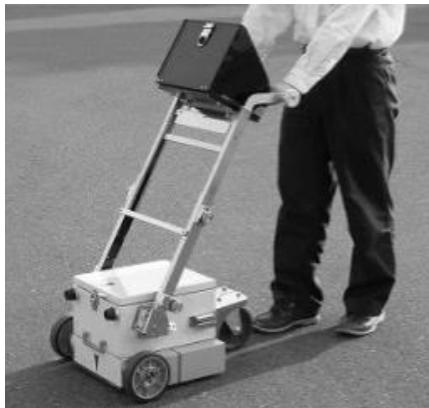
Fig. 3. Configuration of the short-chirp GPR system
